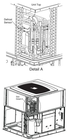
Fig. 27 - Defrost Sensor Location
